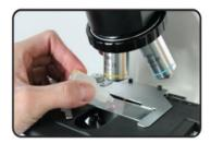
4.5.2 Rotate oil immersion objective(100X) to working position (the objective is marked with oil).
