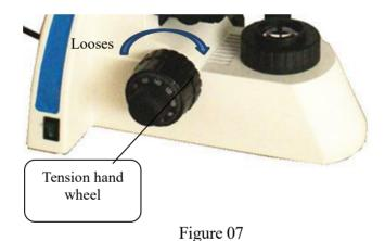
B) For convenience observation and avoid objective to touch with the slider, use stopper when focusing well (figure 07).
