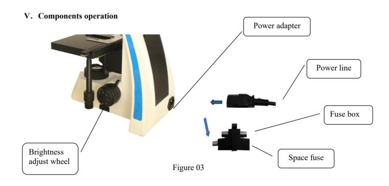
1. Connect power line to host back bottom side. Set illumination knob (on the left bottom side of microscope host) to lowest brightness, rotating illumination brightness by need during operation.
