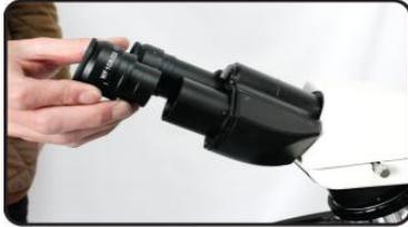
• **Installation of eyepiece and condenser**
