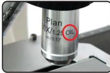
4.5.3 Adjust coarse focusing knob to slowly lift stage until the oil on slide touch bottom face of objective.
