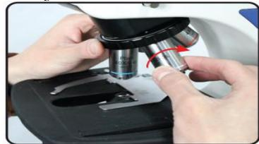
Note: Condenser under stage has been adjusted well, there is no need to install by users again. While need to check its centering in case of shifting during shipment.
