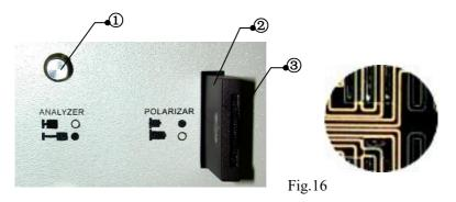
the analyzer and polarizer are orthogonal polarization, the micro-image or field of view is best dark. See fig.16
