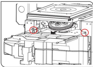
Ⓢ This tray prevents dust, etc. from falling into the microscope.
