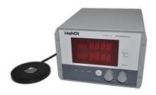
K3000B heating stage is designed for material science, biology and chemical, metallurgical, Polymer and Nanomaterials Science application, it works with optical microscope to observe change and structure during melt, distillation and crystal process. User friendly design is easy to use and stable working to self-adaption fuzzy control.
