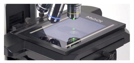
Note: To prevent the thermal plate slipping from the stage, you can install 'Clips' comes with the package to the position 1 and 2 in above image. And clamp the thermal plate by clips.
