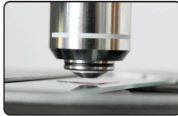
4.5.4 Waggle nosepiece to eliminate bubbles in oil medium, then fix oil objective to make oil full of objective and slide.
