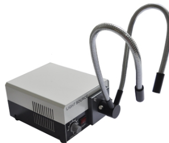
Model: H-150 Fiber light source 21V 150W
