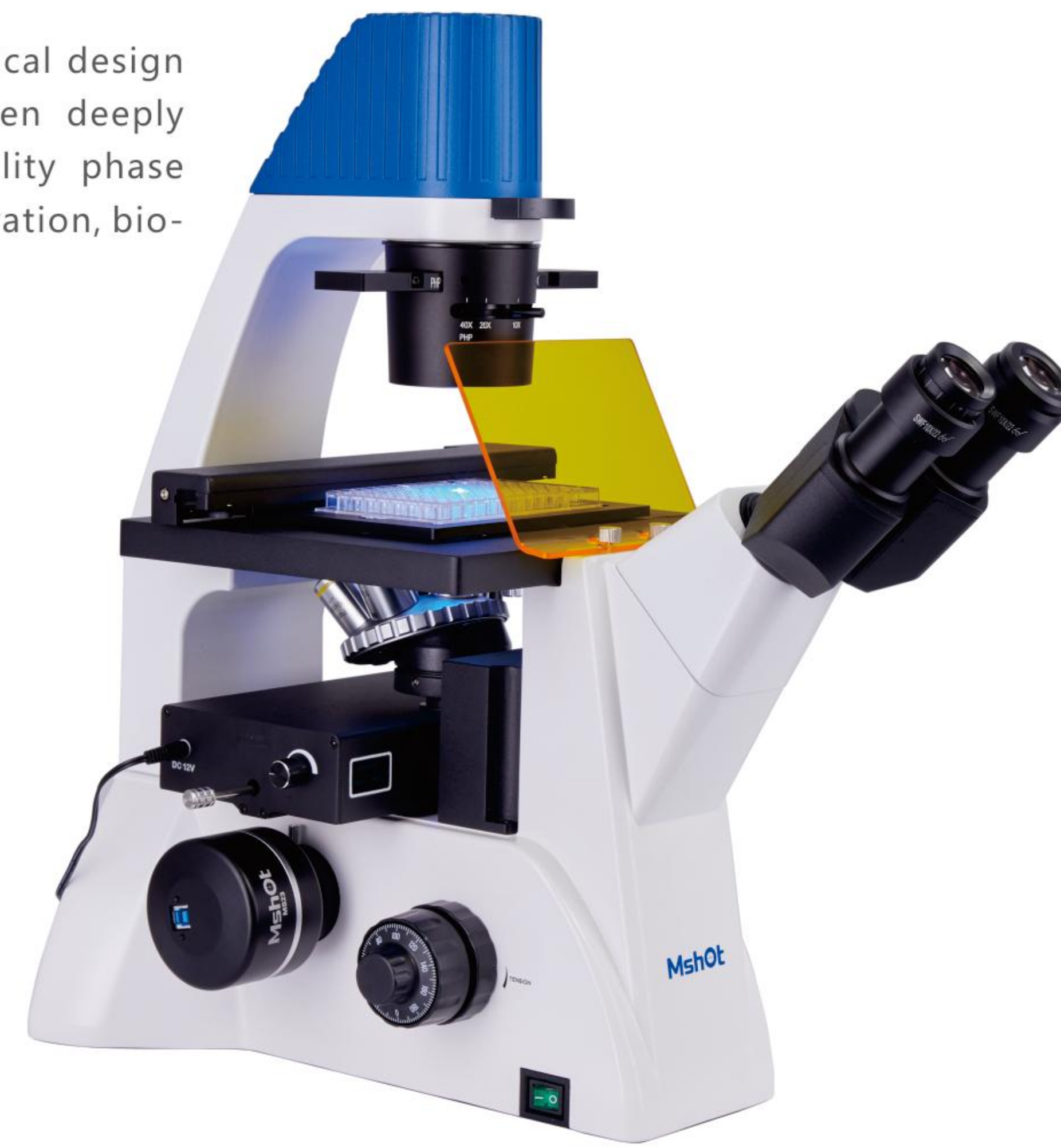
Support phase contrast, fluorescence and bright field observation
