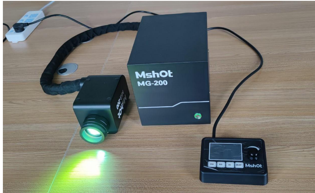
Liquid cooled LED light source Light intensity better than mercury
